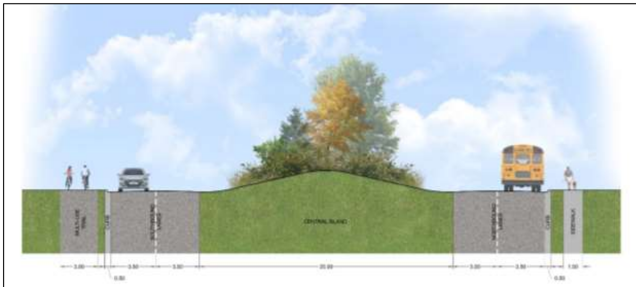
Exhibit 6-6: Elongated Roundabout Section
