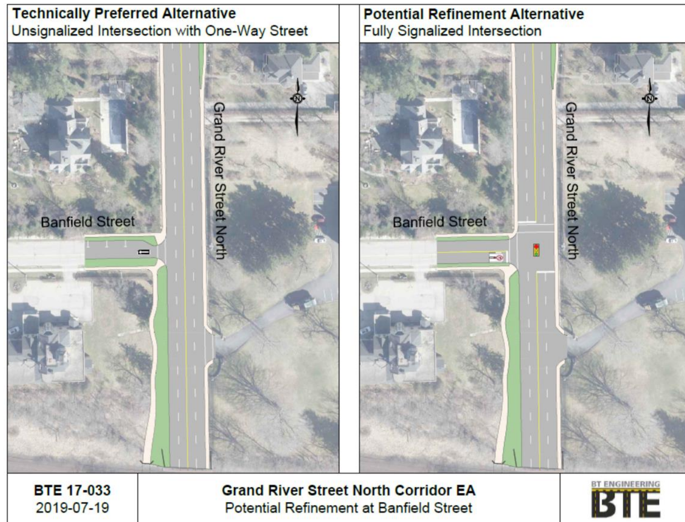
Figure 64: Refinement 4 – Banfield Street Intersection Refinement
