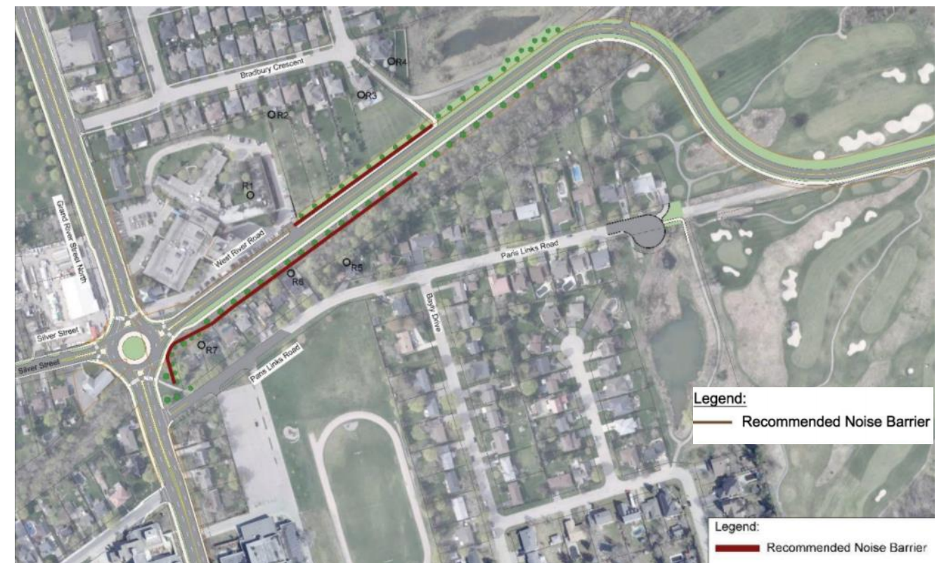
Figure 8: Recommended Barrier Limits and Receiver Sites
