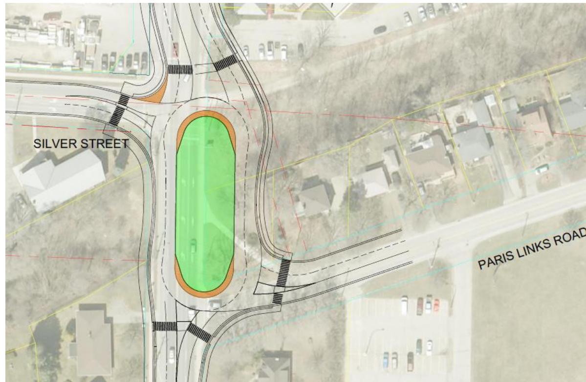
Figure 15: Intersection Alternative ER – Elongated Roundabout
