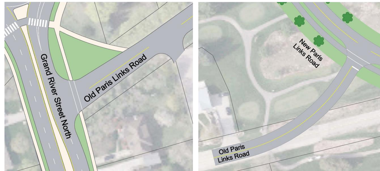
Figure 58: Alternative A – Right-in/ Right-out and T-intersection
