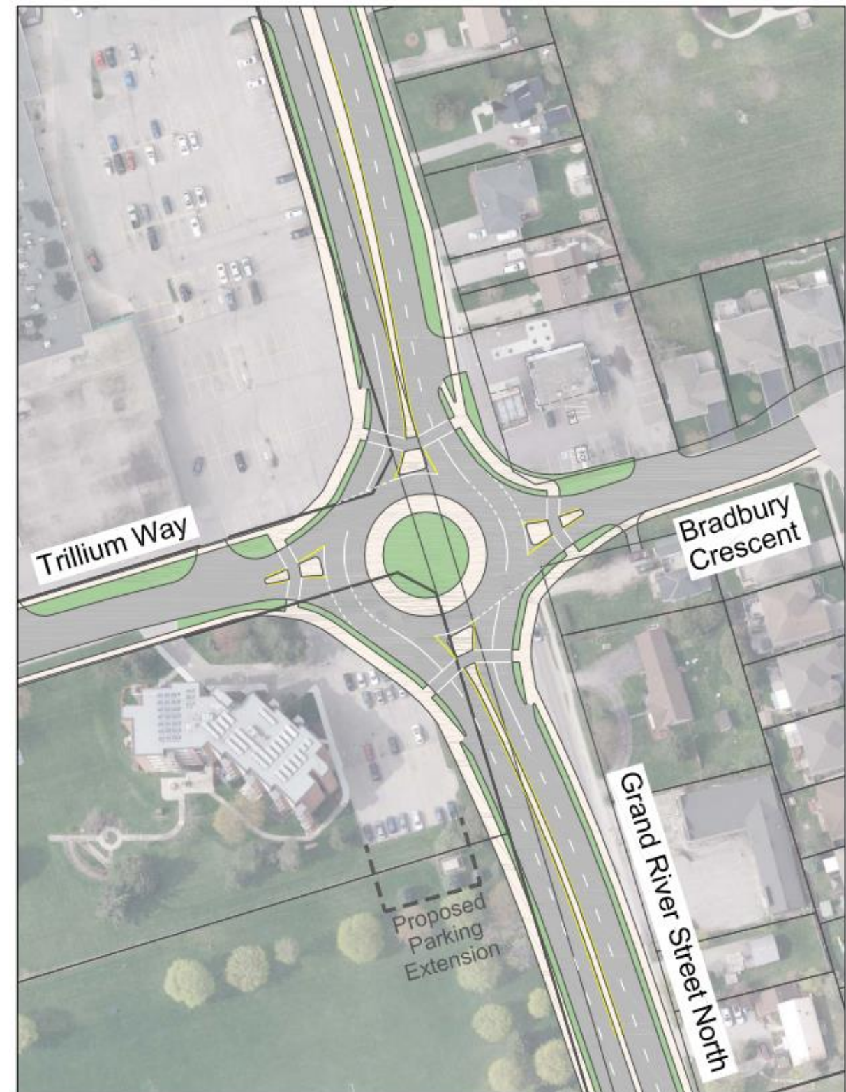
Figure 78: Refinement Alternative C – Shifted Roundabout
