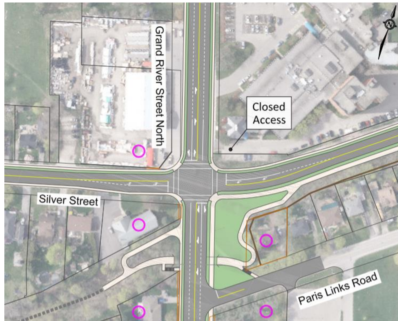
Figure 75: Interim Signalization at Silver Street and Grand River Street North
