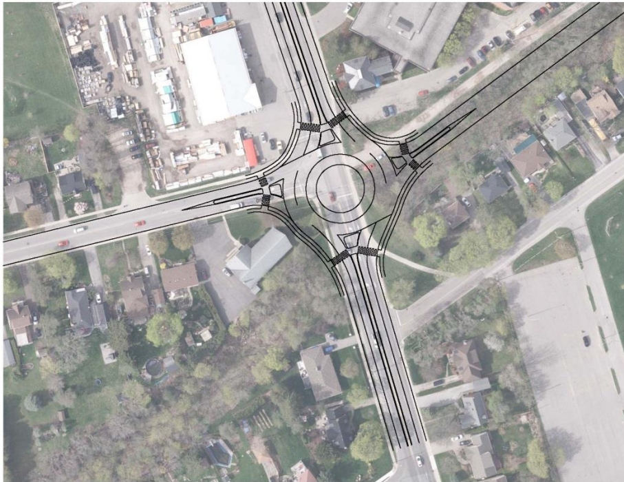
Figure 9: Alternative R - Single Roundabout Intersection
